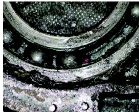
Release Bearing Failure
